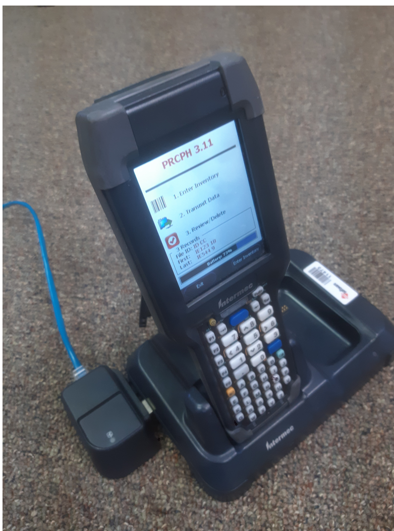
Example of an Ethernet Module Hookup
